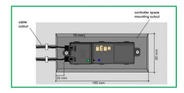
Mounting of controller may require recessed milling to achieve appropriate reading range – Maximum panel thickness 20mm – recommended thickness 10mm. Restrictions for RFID limiting materials apply\*!
