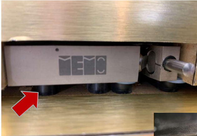
Plastic Lock shims create tension on door.
